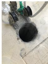
So, I had a go, even rigging up a tripod to separate the deck from the tube, in order to get some fibre glass into the gap. Needless to say, it only worked as a temporary repair and I was on the phone to Andy over Christmas, asking if he could do the job properly for me.
