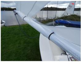
8. Fully hoist the sail and secure the halyard in the cleat. The halyard cannot go in the pocket as it is within the reef, but it can be carefully inserted into rolled sail.
